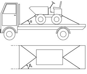
Figure 2 Example of direct lashing
