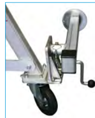
Fig.1 Wind Up Jack Leg in 'parked' position
